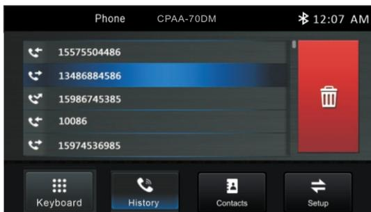
Slide the bar at right side up and down to display a call logs up to 20 records.
