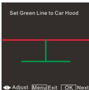
Adjust the DVR position till match the horizon line, press the DVR "up" and "down" buttons, till the lines match. Press "O" button to confirm when finish, will go to next calibration.
