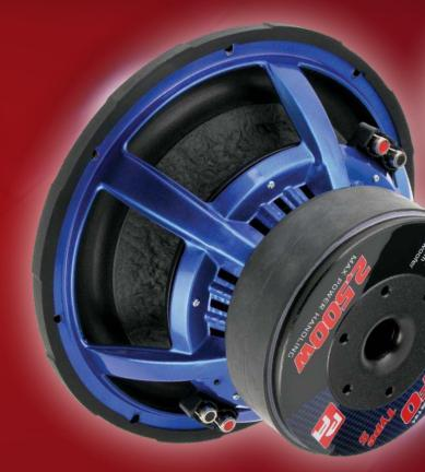
Overcompensating Motor Structure for Maximum Magnetic Strength 10 mm T-Yoke & Top Plate Improve Low Frequency Dynamics Vented T-Yoke & Frame Reduces Voice Coil Heat Build-up Die Cast Aluminum Heatsink Dust Cap Absorbs Voice Coil Heat Aluminum Dust Cap Fins Dissipate Heat & Strengthen Cone 2.5" 4-Layer Voice Coil w/ Large Gauge Wire Increases Power High-Temperature Tolerance Adhesives Resist Thermal Failure
